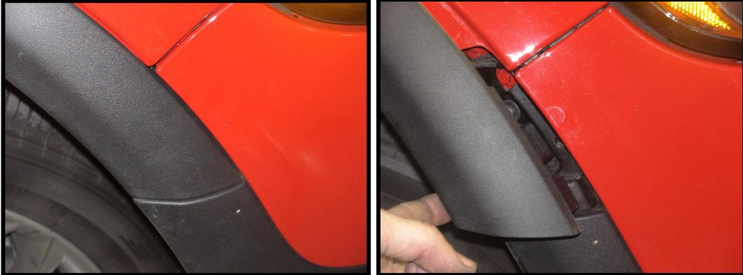
4. Pull away on bumper cover gently and slide off the vehicle as shown:
