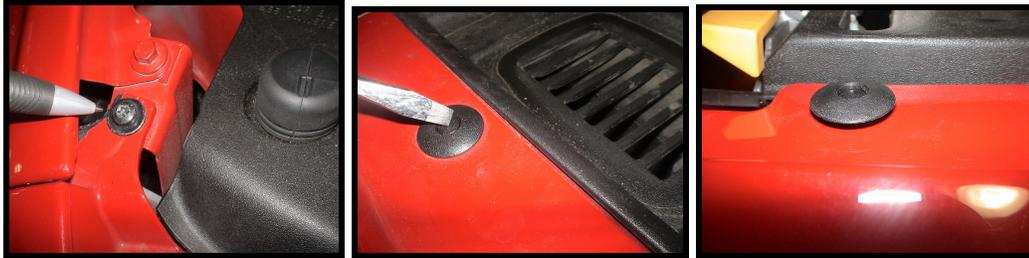
2. Unscrew and remove the (5) screws on the inside of the passenger side fender lining then repeat on the driver side fender lining, behind the bumper cover. Turn the steering wheel to turn wheel/tire as necessary to expose the fender lining. Also, remove lower mounting bolt on each bottom side of the wheel well (as shown on bottom right)
