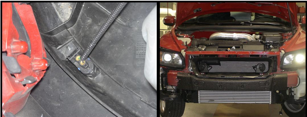
2. Unplug the MAP sensor electrical plug and unscrew hose clamp on both sides of intercooler as shown.
