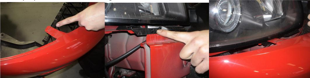
2. Carefully reinsert sides of the bumper cover for proper alignment:
