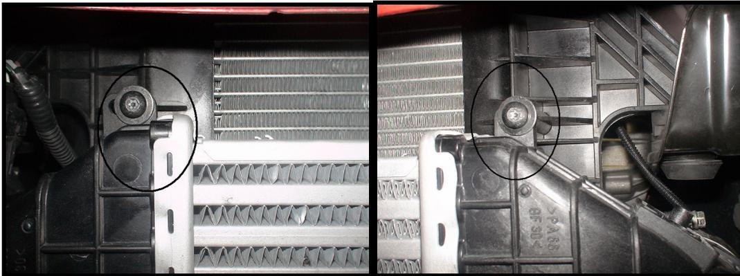
4. Unbolt the MAP sensor from the stock intercooler and slide it into the sensor holder on the ATP intercooler and bolt down using the NEW 4mm bolt provided:
