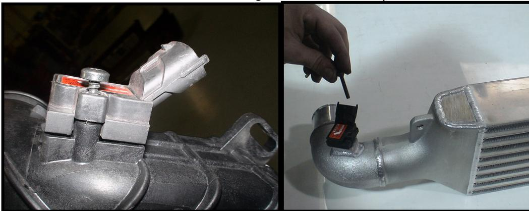
**C. Prepare the brackets and loosely bolt onto intercooler as shown:**
