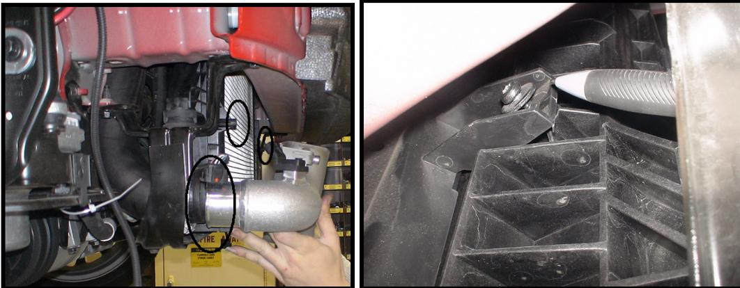
2. Plug the electrical connector for MAP sensor back onto the MAP sensor.
