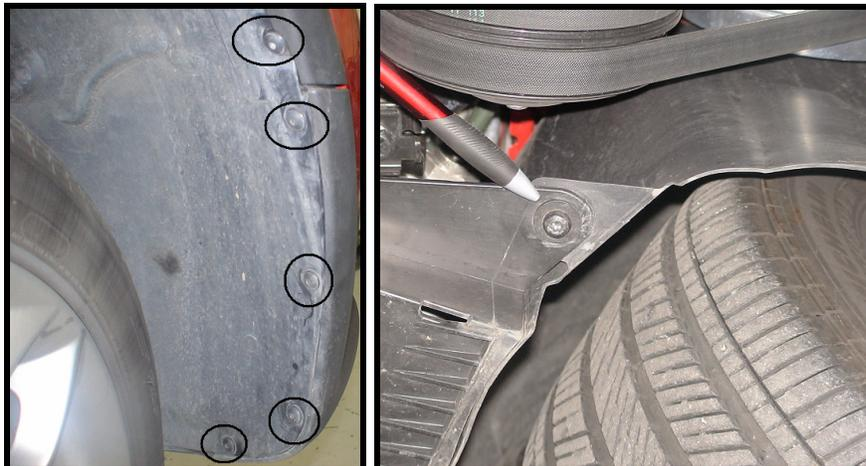
3. Pull away on fender trim away from the front bumper cover as shown. Repeat same process on driver side fender trim.
