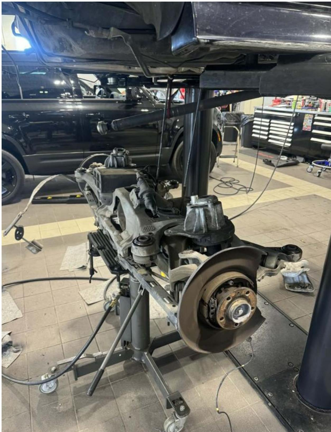
You can use a drill bit to drill several small holes around the bushing which will allow you to easily pry it out
