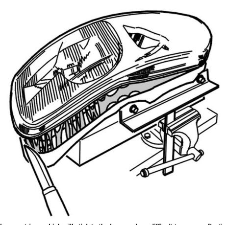
**Note! The adhesive leaves strings which will stick to the base and are difficult to remove.** Pry the glass straight up approximately 5 cm. Start at the side of the outer end. Do not damage the plastic edge on the housing. Lift and hold up the lense.
