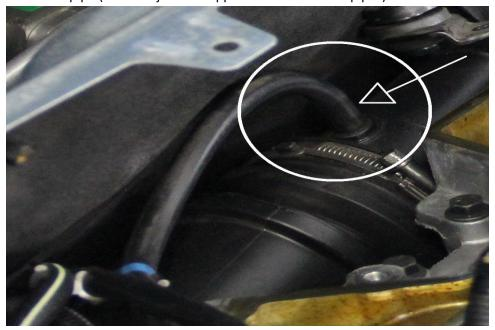
9. Remove the two (2) breather hose clamps from the Crankcase Ventilation Cover (CVC) and upper intake pipe, then remove and discard the short 14mm outer diameter rubber hose that connects the breather box to the intake pipe.
