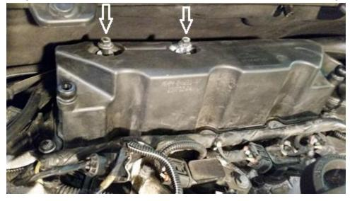
19. Gently tap the front of the CVC with the palm of your hand or a rubber mallet to loosen the gasket seal. Wiggle the CVC front to back, lift up and clear it of the engine bay.
