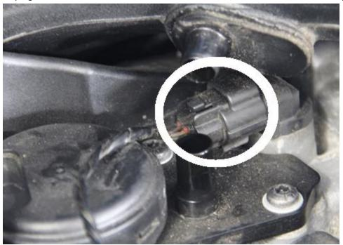
11. On the cam chain side of the engine (right side), remove the one (1) M6 bolt that holds the upper intake pipe to the side of the engine block, and disconnect the electrical connector that is attached to the intake pipe.
