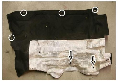
Note: Carefully pull out the insulating cover, being sure not to snag the cover on the metal studs sticking out from the metal panel.
