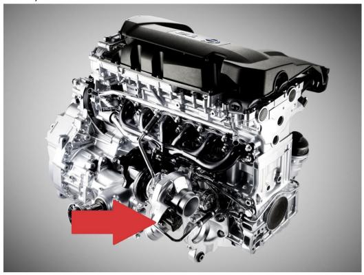
27. You will need to remove the eCRV to install the pCRV. The bolts are hex and a hex key or socket should be used. You will also need to unplug the electrical connector and move it to the side for step 29 below.
