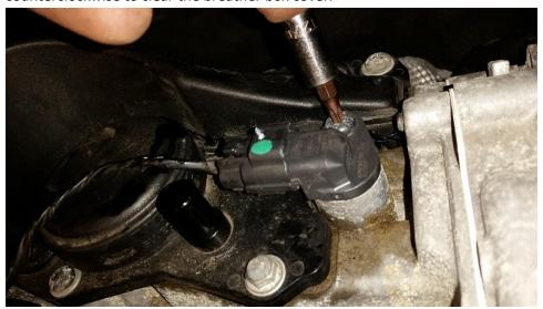
18. Using the T30 bit and a 10mm socket, remove the twelve (12) M6 bolts holding the CVC to the engine.
