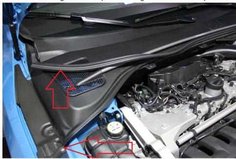
2. If your car has a factory strut brace, remove the honey comb trim panels and the bar itself using a 13mm socket.
