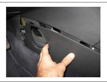
**10.** Remove the plastic trims on both sides of the console, by pulling back and out.
