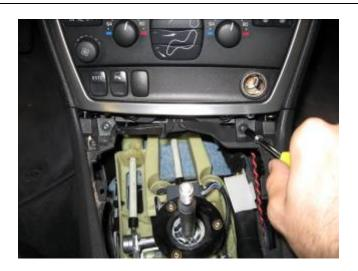
7. Unscrew the two (2) Torx screws at the front of the console, using a T-25 screwdriver.
