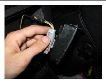
17. Unclip the grey harness by prying it back slightly, and pushing up.
