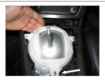
4. Unclip the space ball at front by pulling up. Press the small tab at the rear to unclip the rear of the space ball (if equipped).
