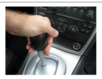
**1.** Remove the shift knob by pushing it down and rotating counter clockwise. Put it aside for re-installation later.
