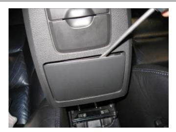
**14.** Using a flat head screwdriver, pry out the plastic cover at the rear of the console.
