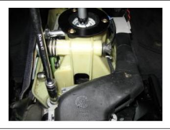
21. Unscrew the four (4) base bolts using a ratchet, a ratchet extension and a 10 mm socket.
