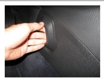
**9.** Unclip the foot well vents on both sides of the center console.
