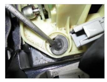
**23.** Using a flat head screwdriver, push out the rubber bushings.
