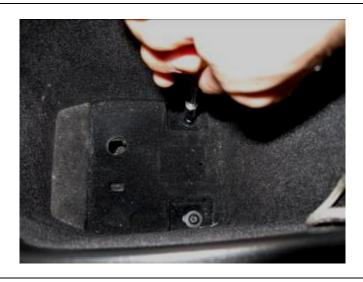
**6.** Unscrew the two (2) Torx screws at the bottom using a T-25 screwdriver.
