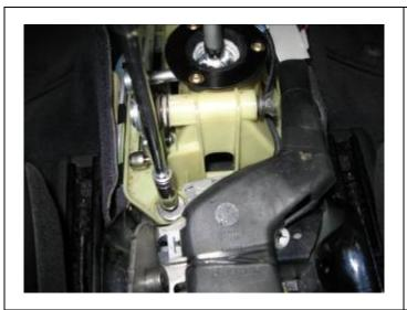
25. Tighten down the TWM assembly with the four (4) included washers and the four (4) stock bolts using a 10 mm socket and a ratchet.
