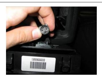
**16.** Unclip the black circular wire by pulling it out of its holder.
