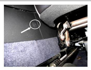
8. Locate the slotted caps on both sides of the console. You will have to move the seats all the way back. Use a quarter to rotate it 90° counter clockwise.
