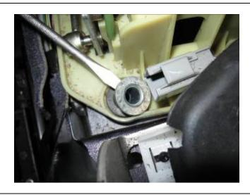
**22.** Using a flat head screwdriver, pry the metal sleeve out of the rubber bushings.
