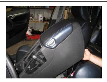
13. Pull up the rear of the center console. This will make the next steps much easier. Be careful not to scratch the radio layout.
