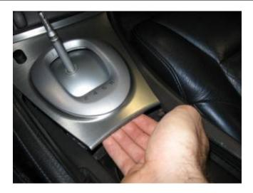
**3.** Pull up on the silver portion of the center console. The back part will unclip first, then you can work your way underneath the console to unclip the front.
