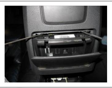
**15.** Using two screwdrivers, pry out the plastic housing behind the cover unclipped at step 14. This will free both plastic components.
