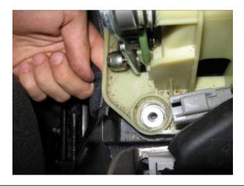
**24.** Slide the TWM base bushings under the stock shifter.
