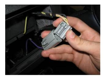
**18.** Unclip the two parts of the grey harness by pressing down on the tab at the top.
