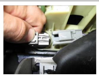
20. Unclip the grey harness above the rear left base screw. This wire controls the reverse lockout solenoid (if equipped).
