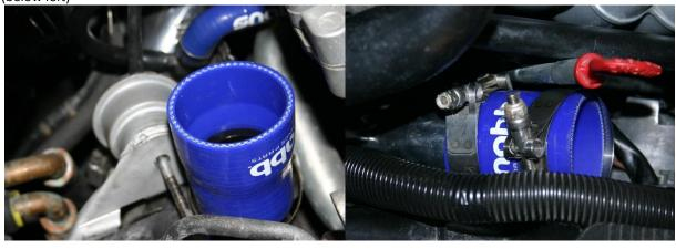
Install the 2.25" straight coupler to the top of the lower IC inlet pipe with a supplied 2.56" Tbolt, tighten all the way. (Above right)
