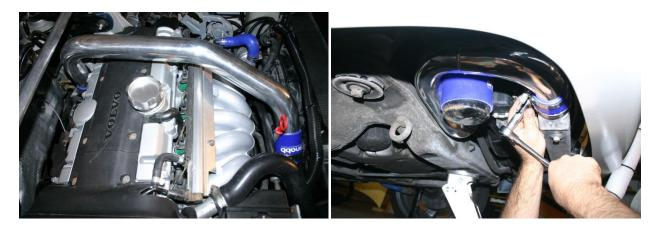
Install upper IC inlet pipe into the two silicone couplers along with 2.56" t-bolts on each side. Position the Tbolts as shown and tighten down all the way if everything is aligned correctly. If not, reposition as needed then, tighten clamps. Now go back and finish tightening the bottom IC inlet clamps that you left loose. (see above)
