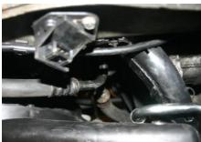
Also note that if you have a 98 you will want to temporarily unplug the sensor shown in the picture above that is mounted to the sub-frame.
