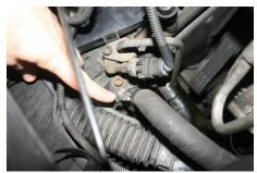
Next loosen the mounting screw (see above right) on the top of the dryer and angle the bottom of the dryer towards the front of the car as much as you can and then retighten the bolt.
