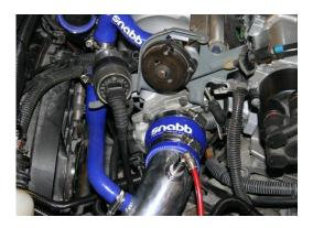
Next install the Lower Idle air control motor hose to the FMIC piping. The motor may need to be rotated slightly or the IC pipe may need to be moved closer to the throttle body for this to fit on. Tighten with the small (included) worm clamps. (above right)
