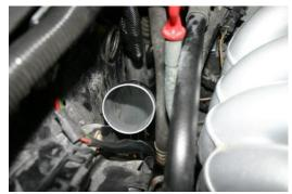
Next slip the pipe up through the opening where you trimmed the plastic tab earlier. (see above) You may need someone to help you with this as the power steering lines can get in the way when you are trying to push the pipe up into the engine bay. The pipe needs to be rotated slightly as shown and installed up from the bottom at an angle in order to get it into position.
