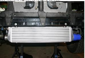
**Trim plastic tab** off bottom passenger side of radiator shroud by the bottom oil cooler bend as seen in picture. Additionally you will need to remove the small rubber flaps that are mounted to the back of the fan shroud (if your car still has them)
