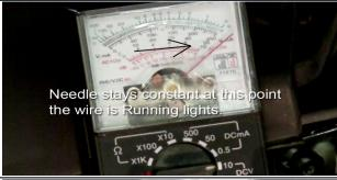
If the needle bounces on the meter, the wire is a turn signal. The voltage to the turn signal pull high and low in order for the turn signal to blink.
