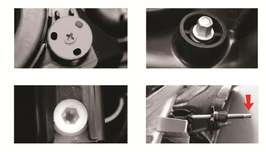
Next locate the tools that will be needed to adjust your headlamps. Note: Please do not ever use power tools on your adjusters this may cause severe damage to the internals of your lights.
