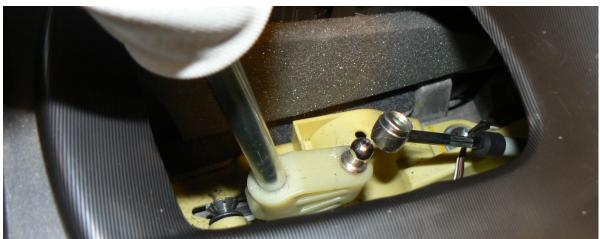
2. Place both parts of the adapter onto the shaft just under the boot where it can be easily reached. (Make sure that the alignment of the small piece is correct as it is not perfectly symmetrical: You want the back edge of the two pieces to be flush when mounted on the shaft so that the bolts align correctly and do not get cross threaded) Thread the (4) bolts by hand until they are mostly in but still loose enough that you can slide the adapter down on the shaft.
