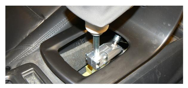
\*\*Please note that raising or lowering the adapter on the shaft will slightly alter whether the shift lever is perfectly straight up and down. For this reason there is a small amount of adjustment available on the ball location. For example: If you find that the shifter is slightly forward you can remove the ball with ½ drive socket and wrench and move the ball reward to straighten the shift lever and vice versa. There is approximately 1 inch (shift knob travel) of total adjustment available.
