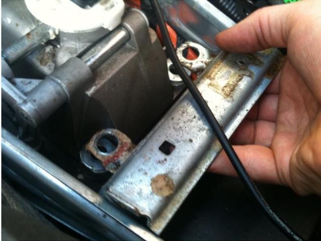
4. Remove the rubber bushings and metal inserts from the shifter assembly.
