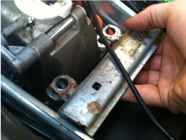
3. Remove the rubber bushings and metal inserts from the shifter assembly.
