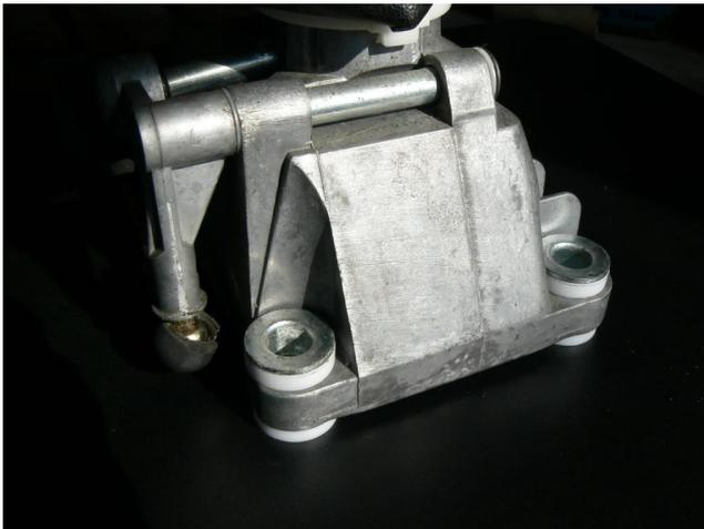
7. Place the small horizontal metal bracket back over the rear of the assembly and reinstall the side bolts first tightening partway. Next reinstall the bolts that hold the assembly down: Apply locktite to the bottom of the bolts and tighten down while keeping the washers and metal inserts centered under the bolts. Tighten the side bolts.
