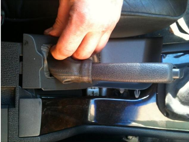
3. Pull up on the base of the shift boot to separate it from the console trim.
