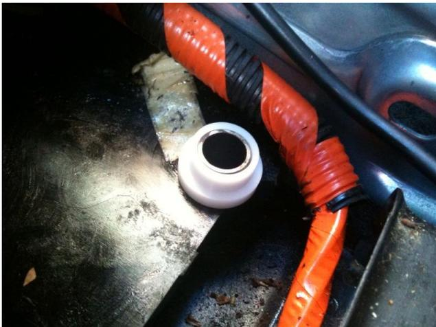
5. Place the assembly over the spindles and new bushings then place the set of Delrin washers on top of the holes. Place the metal inserts in through the washer.
