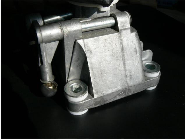
6. Place the small horizontal metal bracket back over the rear of the assembly and reinstall the side bolts first tightening partway. Next reinstall the bolts that hold the assembly down: Apply locktite to the bottom of the bolts and tighten down while keeping the washers and metal inserts centered under the bolts. Tighten the side bolts.
