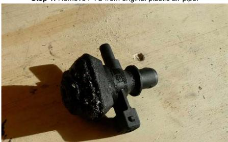
**Step 1:** Remove PTC from original plastic air pipe.
