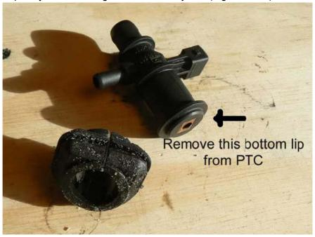
The PTC can now be installed into the SNABB metal piping!
